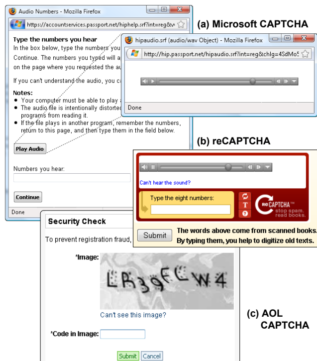
Figure 1. Examples of existing interfaces for solving audio CAPTCHAs. (a) A separate window containing the sound player opens to play the CAPTCHA, (b) the sound player is in the same window as the answer box but separate from the answer box, and (c) clicking a link plays the CAPTCHA. In all three interfaces, a button or link is pressed to play the audio CAPTCHA, and the answer is typed in a separate answer box.
